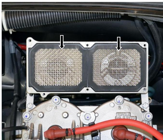
Inspect gasket. Replace if damaged or brittle.
