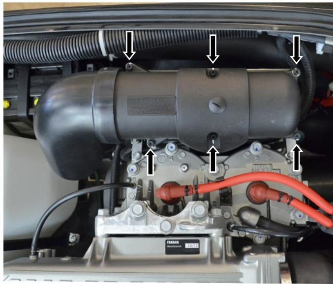
Remove stock air intake cover mounting plate (6 bolts).
