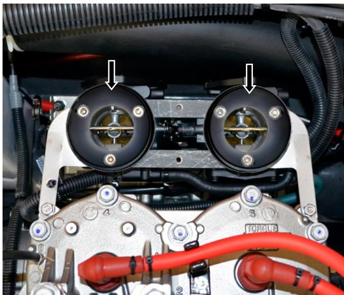
**TIP: Place bolts into adapters and then carefully place adapters onto carburetors!**
