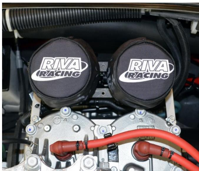
Install Power Filters onto carburetor adapters and secure.
