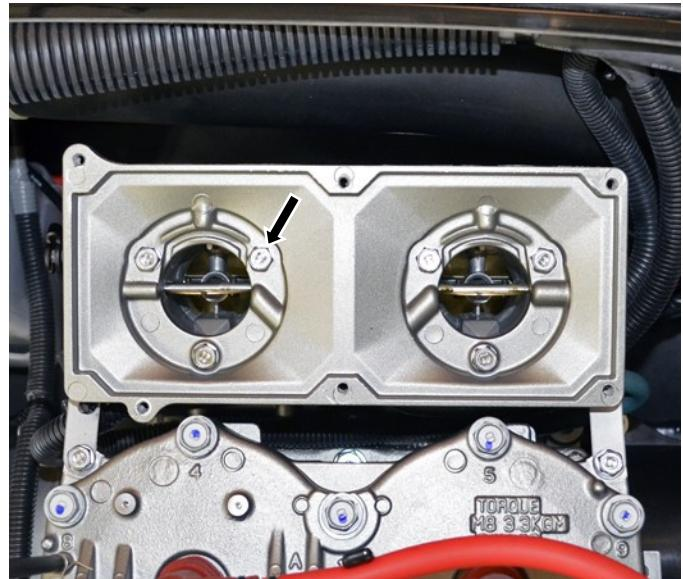
Remove internal spark arrestor screens (2) and discard.
